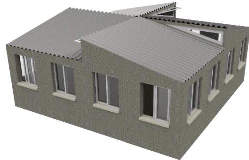
F6 – Cross Ventilation Scheme with added roof windows in a 0.3 glazing ratio house (south-eastern perspective view).
